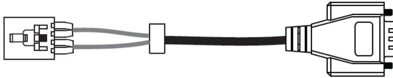
**Optional Video Connector Kit Assembly for SB800 Series (Part No. 20-01496-20)**
