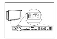
2. Press the **Input Select** button on the interactive flat panel's front control panel until the input source is *HDMI1*.
