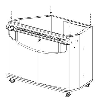
10. Using the hex key provided in the accessory kit, insert and tighten two of the four supplied security screws to the underside of the top cabinet, on either side of the pen tray.
