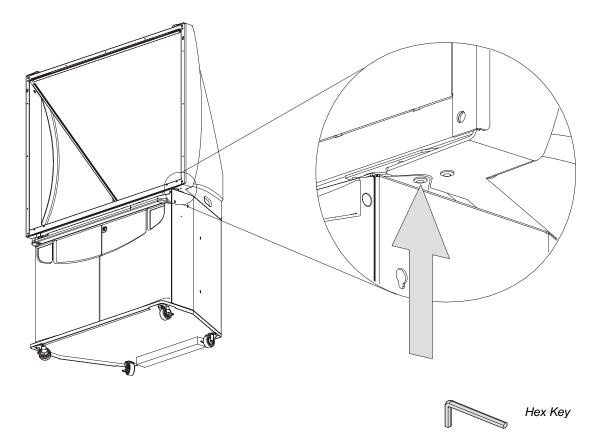
11. Using the same hex key, secure the remaining two security screws inside each side handle.
