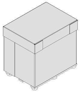
2. Remove the band that holds the pallet ramp against the touch screen. Lower the pallet ramp.
