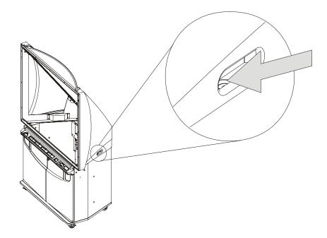
12. Before attaching the screen, remove the protective cardboard liner from the back of the screen. Then, with each person holding the screen by the top and bottom corners, carefully hang the screen by inserting the two upper-corner standoff posts into the corresponding keyholes on the cabinet.
