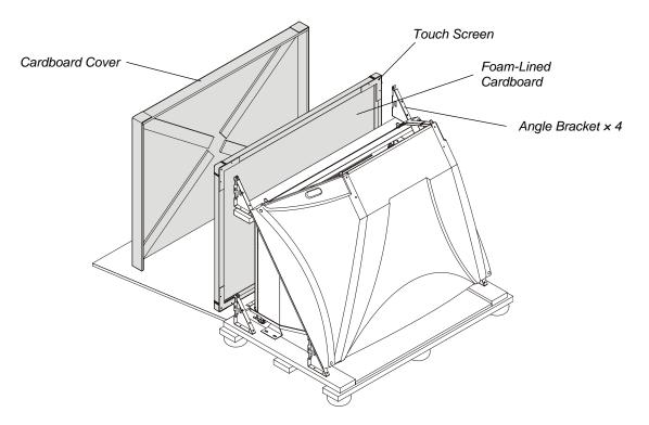
5. Using a Phillips® No. 2 screwdriver, loosen the four captive corner screws that secure the cabinet top to the angle brackets.
