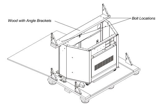
8. Using the 9/16" wrench provided (you'll find it attached to the pallet) remove the bolts that secure the four orange shipping brackets that hold the bottom half of the cabinet to the pallet. You can also remove the four angle brackets from the pallet, if necessary. You can now wheel the lower cabinet down the pallet ramp.
