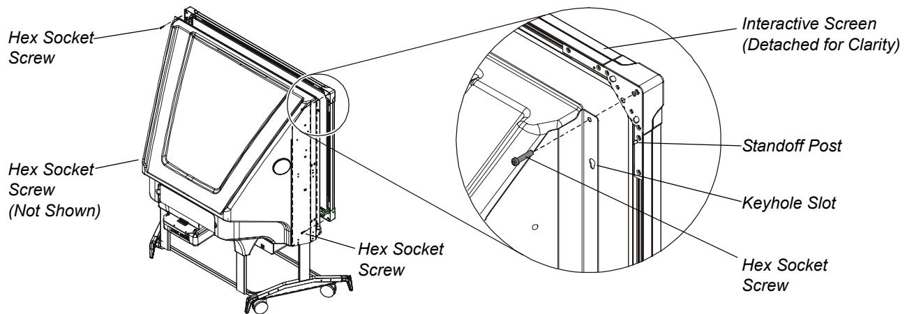
6. With the screen still suspended on its standoff posts, pull the right bottom corner of the screen (as you face the front of the 2000i) a little away from the cabinet, and reach inside to disconnect the modular cable and the power cable from the Communications Hub at the back of the screen.
