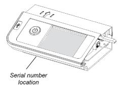
The appliance serial number is located under the power button of the appliance.
