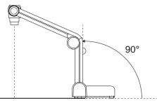
4. Rotate the upper arm of the document camera upwards until it's at its highest spot, ensuring the bottom arm is still set to 90°.
