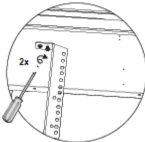
5. Repeat steps 3 and 4 for the right rack rail, except rotate the rail counter-clockwise before inserting it into the rack mount slots.
