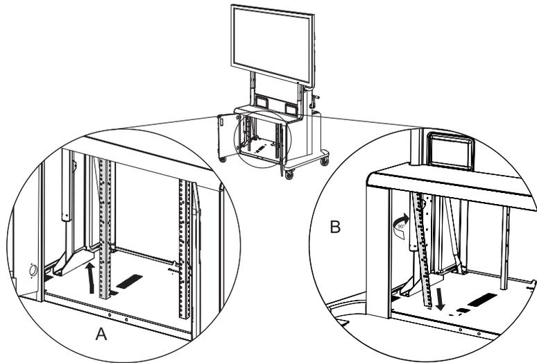
4. Straighten the rack rail, aligning the holes in the flange at the top of the rail to the pilot holes in the cabinet's top panel, and then secure the rail with two of the screws that you removed step 2.
