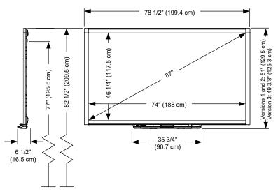
Leave at least 5/8" (1.6 cm) headroom to wall mount the SB885. The distance from the bottom of the wall mount bracket to the top of an installed interactive whiteboard is 6 1/8" (15.6 cm)
