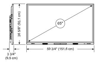
Weight 34.4 kg Shipping dimensions (including pallet) 142.3 cm × 90.4 cm × 23.5 cm Shipping weight 51.1 kg VESA mount M8, 400 × 400 mm Handles 2
