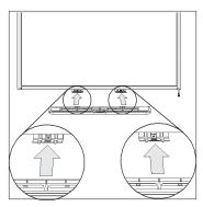
5. Route the modular I<sup>2</sup>C cable through the cable management channel under the lower-right end of the pen tray, and then insert its connector into receptacle 1.
