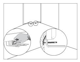
2. Remove your interactive whiteboard from the wall, and then use the screwdriver to secure a self-tapping wall anchor at each mark.
