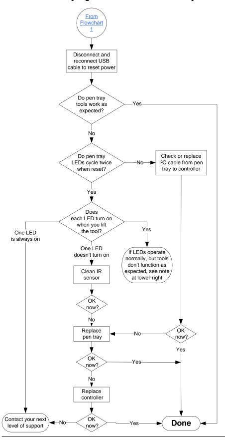
When you disconnect and reconnect the USB cable to reset the power, all of the pen tray LEDs flash sequentially twice, indicating successful communication with the controller. If they flash continuously, contact your next level of support.
