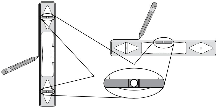
All of the lines that you draw to install the SB600i3 must be straight and level on a plumb wall. You must install the unit straight, level and plumb for it to operate properly.
