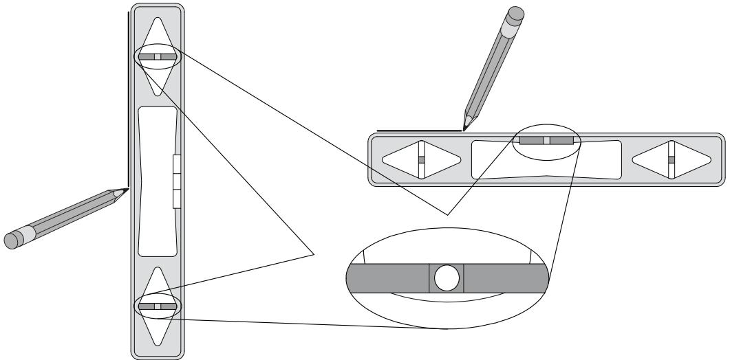
All of the lines that you draw to install the SB600ix must be straight and level on a plumb wall. You must install the unit straight, level and plumb for it to operate properly.
