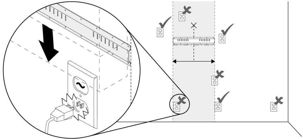
If you need to attach a peripheral device, guest computer or laptop to the interactive whiteboard system, make sure that the cable is long enough so that, at this highest or lowest height, the HAWM-UX/UF doesn't pull the laptop or peripheral.
