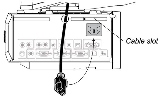
2. Place the power cable around the back of the HAWM-UX/UF toward the left side of the interactive whiteboard if the power outlet is located on the left, or toward the right side of the interactive whiteboard if the power outlet is located on the right.
