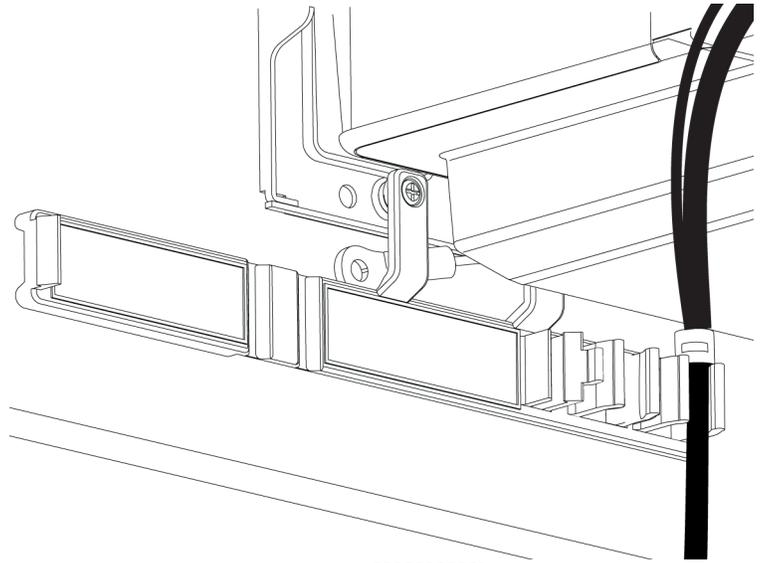
3. If the ECP is mounted on the left, place the WMB around the back of the HAWM-UX/UF's interactive whiteboard brackets, toward the left side of the interactive whiteboard. If the ECP is mounted on the right, place the WMB around the back of the HAWM-UX/UF's interactive whiteboard brackets, toward the right side of the interactive whiteboard.
