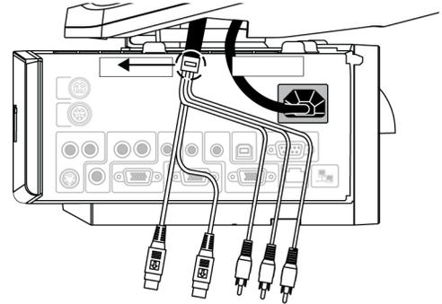
2. From the ECP harness cable, attach the composite video RCA jack, its associated dual channel audio input (two RCA jacks), the 4-pin power mini-DIN connector and the 7-pin mini-DIN connector to the projector's connection panel.
