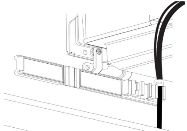
3. With the ECP mounted on the left, place the WMB around the back of the HAWM-UX/UF's interactive whiteboard brackets, toward the left side of the interactive whiteboard for proximity to the ECP.
