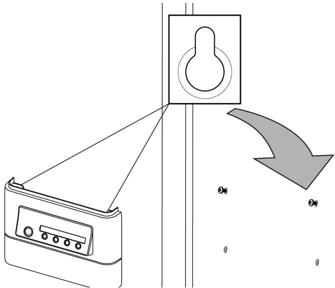
10. Flip up the bottom panel of the ECP. Attach two screws in the two bottom plastic anchors using a Phillips No. 2 screwdriver.
