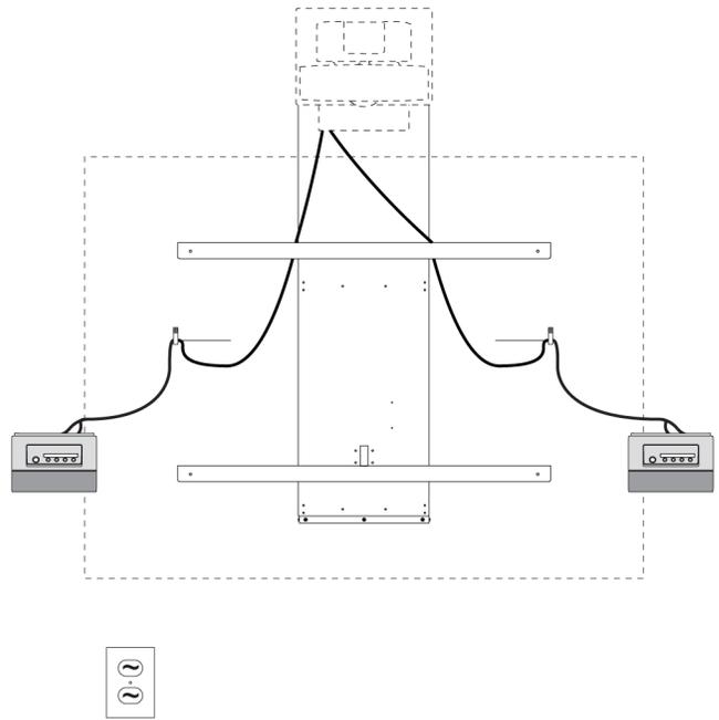
9. Attach a cable management clip (not included) to the cables or cable bundles, making sure there's a minimum of 28" (71.1 cm) excess straight length or a 14" (35.6 cm) loose loop of cable.
