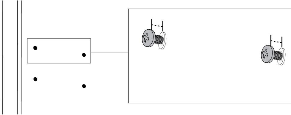
9. Attach the ECP to the screws, using the top two key holes on the ECP.
