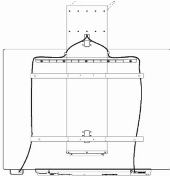
7. Attach the cables to the lower cable clips on the HAWM.
