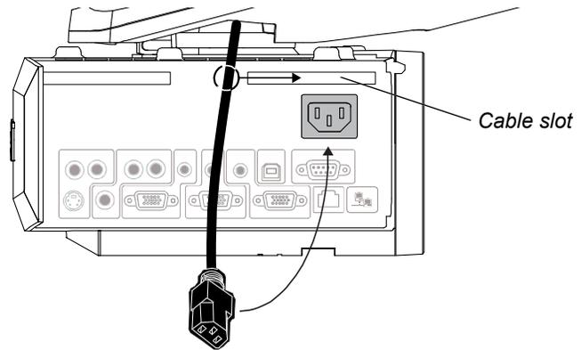
2. Secure the power cable to the SMART UF65 or SMART UF65w projector's wall-mount bracket using a cable tie. Place the cable through the cable cutouts on the wall-mount bracket.
