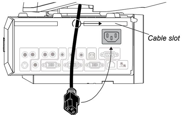
2. Secure the power cable to the SMART UF55 or SMART UF55w projector's wall-mount bracket using a cable tie. Place the cable through the cable cutouts on the wall-mount bracket.
