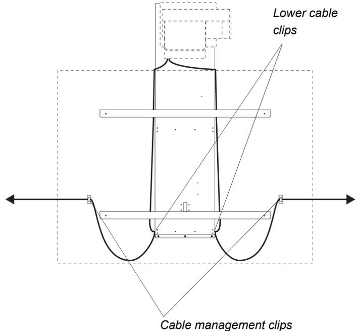
6. Attach the cables to the lower cable clips on the HAWM-UX/UF. If you have many cables attached, smoothly bundle your peripheral device cables together using a cable tie (not included).
