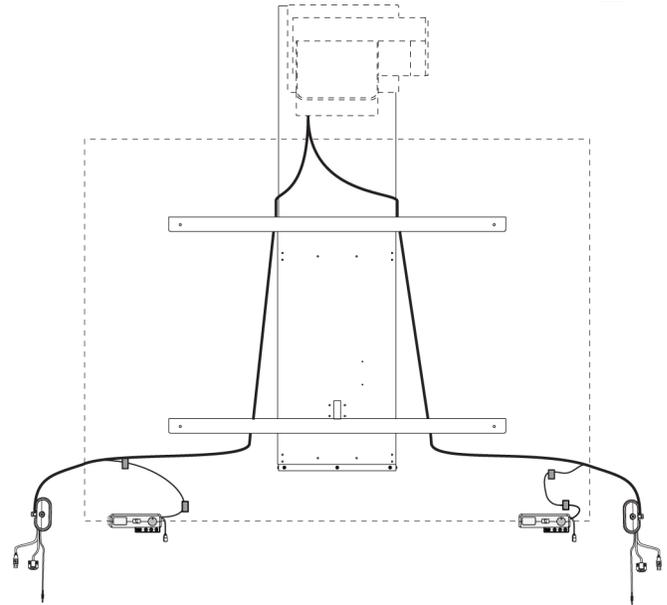
4. Place the WMB through the top cable clip you installed on the side of the HAWM-UX/UF.
