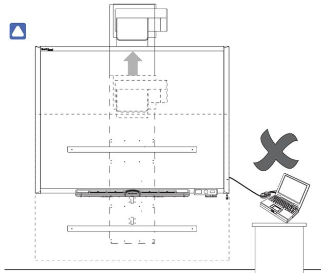
Mount your peripheral devices to a permanent location near the HAWM-UX/UF. If the peripheral device moves or can move, it can cause cable strain if the device is moved too far from and interferes with the HAWM-UX/UF.
