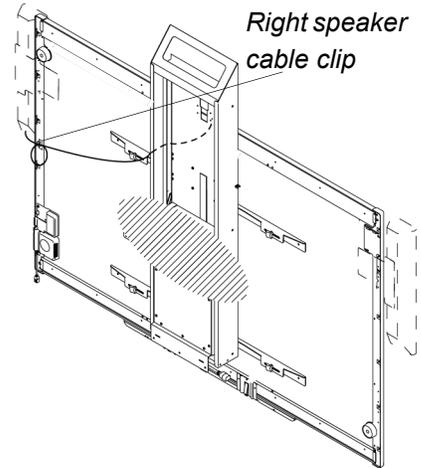
7. Place the Molex cable through the left speaker cable clip, through the space between the HAWM-UX/UF and the interactive whiteboard.
