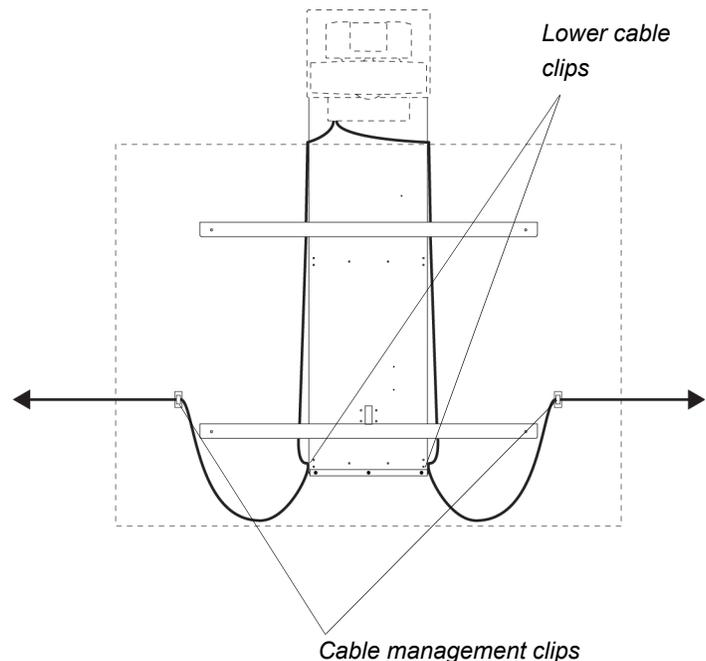
8. Attach the cables to the lower cable clips on the HAWM.
