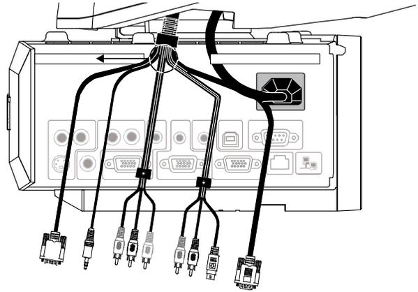
3. Connect the S-Video connector and two audio-left/right RCA jacks, the DB9 control cable and the composite video and two audio-left/right RCA jacks, from the ECP harness cable, to their receptacles on the projector's connection panel.
