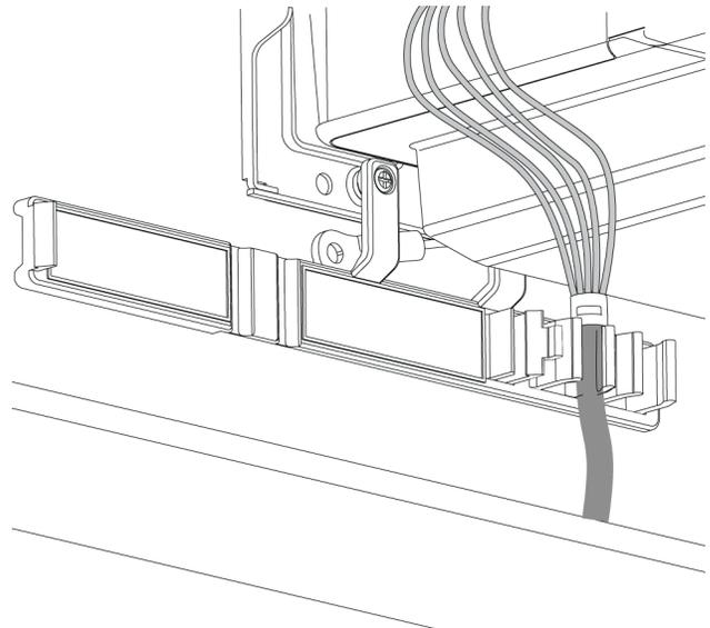
3. Place the harness cable around the back of the HAWM-UX/UF's interactive whiteboard brackets toward the left side of the interactive whiteboard if the ECP is mounted on the left or toward the right side of the interactive whiteboard if the ECP is mounted on the right.
