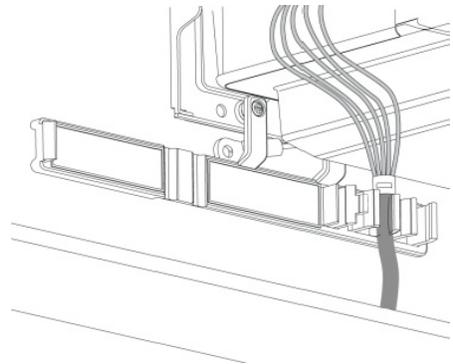
3. Connect cables from the projector to the interactive whiteboard, making sure that all cables pass between the two interactive whiteboard wall-mounting brackets. Once the cables are through the brackets, place the harness cable toward the left side of the interactive whiteboard for proximity to the left-mounted ECP.
