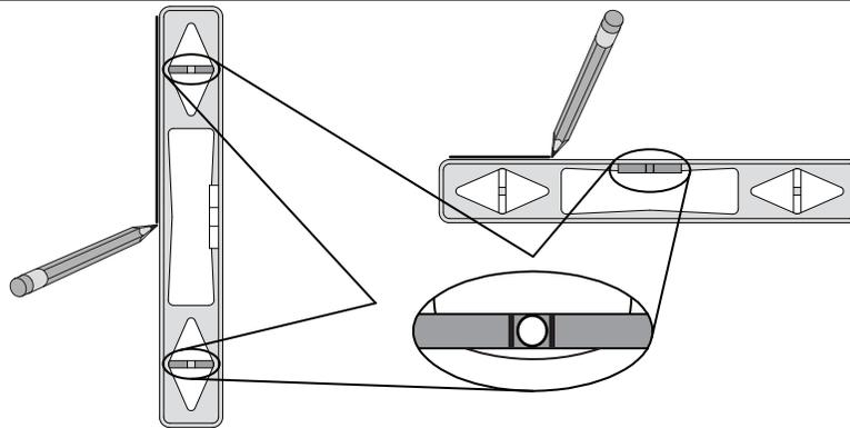
All of the lines that you draw to install the SB600i5/SB600i5-MP must be straight and level on a plumb wall. You must install the unit straight, level and plumb for it to operate properly.
