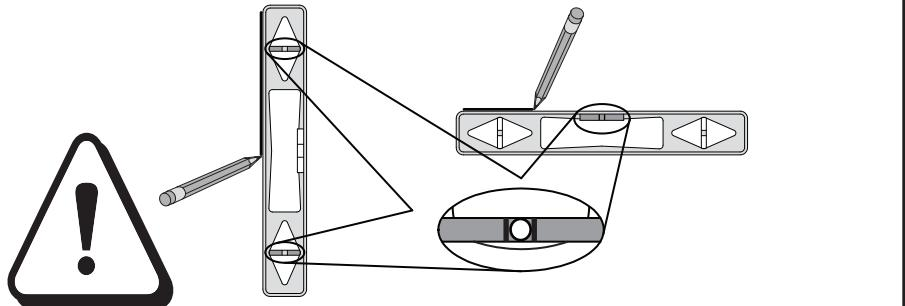
All of the lines that you draw to install the SB800ixe-SMP must be straight and level on a plumb wall. You must install the unit straight, level and plumb for it to operate properly.
