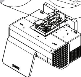
Fully insert the projector adjustment module into the wall mount bracket guide pins. You will hear a click when the adjustment module is fully inserted and the spring is locked. Refer to step 3 to safely secure the system using the three locking screws.
