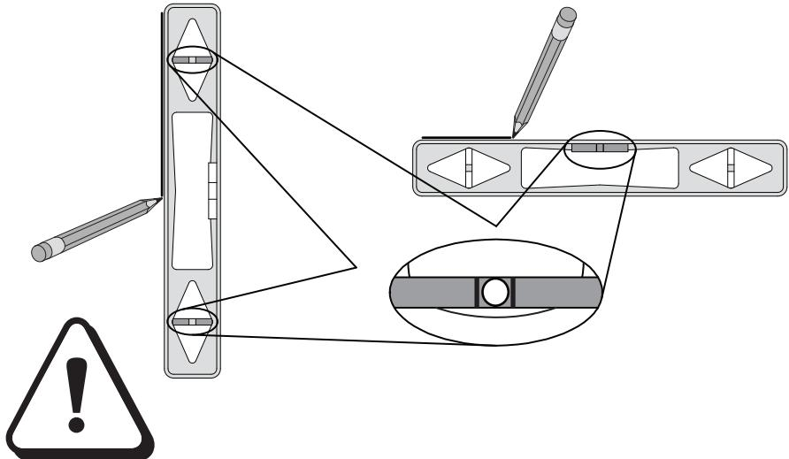
All of the lines that you draw to install the SB800i5e-SMP must be straight and level on a plumb wall. You must install the unit straight, level and plumb for it to operate properly.
