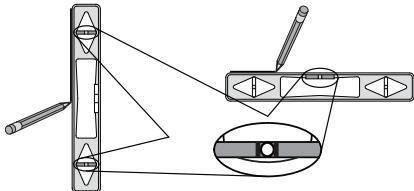
All of the lines that you draw to install the SB800i5 must be straight and level on a plumb wall.
