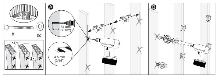
**CAUTION:** This wall mount or stand is intended for use with a display system with a maximum weight of 276 lb. (125 kg) and a maximum diagonal of 84" (214 cm). Use with products that are heavier than the maximum weight indicated may cause the mount and its accessories to collapse, resulting in possible personal injury.
