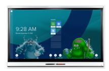
The 65" 4K ultra-high-definition LED display provides optimal image clarity and wide viewing angles. With the Pen ID™ feature, you can assign different appearances to the two pens and write or draw over any application in digital ink.
