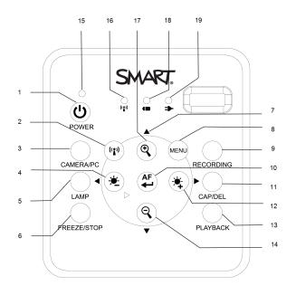
The control panel to enables you to switch between Camera, Computer Pass-Through, and Playback modes. Additionally, using the control panel allows you to adjust the settings and features in the Camera mode's on-screen display (OSD) menu.
