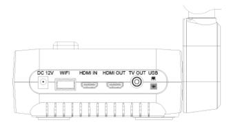
The rear panel of the document camera consists of the following connectors:
