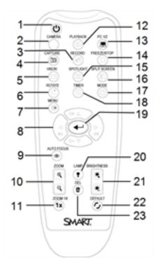
All features of the SMART Document Camera 550 can be accessed with the remote control. The remote control requires two AAA batteries.
