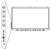
The convenience panel contains buttons for turning the display on and off, controlling the volume, freezing and unfreezing the screen, and showing and hiding a screen shade. It also includes connectors for USB peripherals and a computer or other input source.
