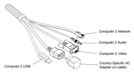
2. If necessary, connect the country-specific power adapter to the end of the AC power cable.
