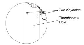
2. Push the two protruding bolts on the edge of the shelf into the two keyholes, and then push the shelf firmly down.
