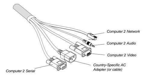
2. Connect the Computer 2 Video cable from the laptop cable harness to the **Computer 2 Video IN** (female) connector on the connection panel.
