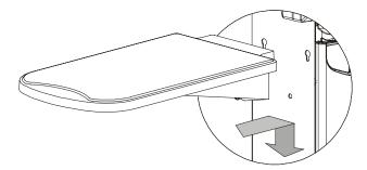
3. Push the captive thumbscrew at the bottom of the shelf into the thumbscrew hole and tighten.
