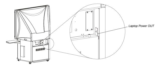
If the **Laptop Power OUT** connector is located below the connection panel and *behind* the rear access panel, perform the following steps.
