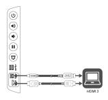
After you've connected computers and other input sources to the display, switch between these input sources by showing the Home screen, tapping **Input**, and then selecting an input source.
