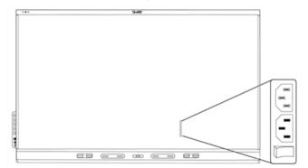
There is a power switch on the back of the display next to where the power cord plugs in.
