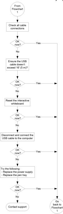
A red Ready light indicates that the interactive whiteboard is receiving power but isn't communicating successfully with the computer. In most cases, pen tray lights don't turn on and the screen doesn't respond to touch.
