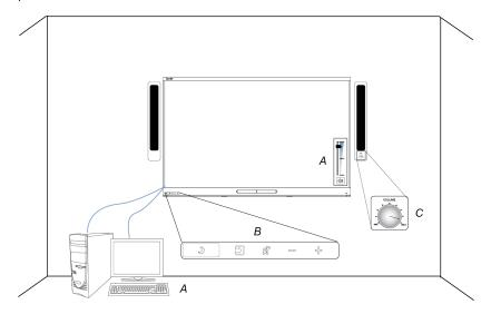
**A** Audio signal source (a media player on the computer connected to the display)
